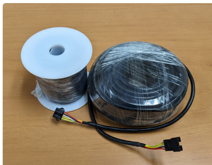
Modbus wire (left) and display wire (right)
