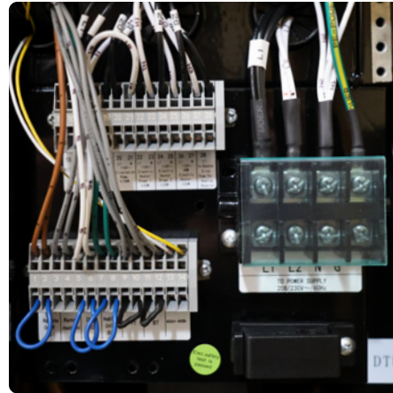
CC32-18 electrical connections.
