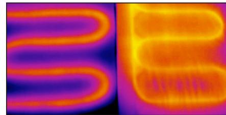
After 2.5 hours, gypsum concrete is producing 10 BTUs/sf, while Warmboard is producing 18 BTUs/sf, with more even surface temperatures. The variation in temperature across the surface of Warmboard is only 2+°F while gypsum concrete has 6°F of variation.
